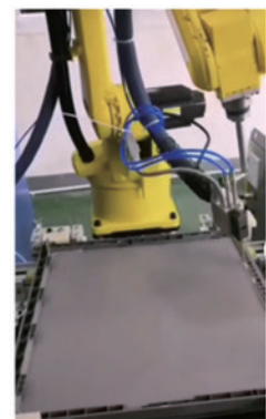
Gluing of control cabinet doors
