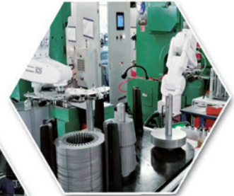
Handling of Motor Stator Silicone Steel Sheets
