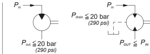
The Motors are equipped with HPD shaft seal (20bar), on request is available also for motor with outrigger bearing.
